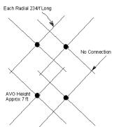
Fig 2—Elevated radials (top view).
